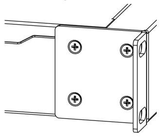
The device is designed to use indoors and it can be mounted in a rackmount enclosure using provided rack mounts, or it can be placed on the desktop. Please attach rubber pegs on the bottom of the router if the desired placement is on the flat surface or use a Phillips screwdriver to attach rackmount ears on both sides of the device if designated use is for rackmount enclosure.
