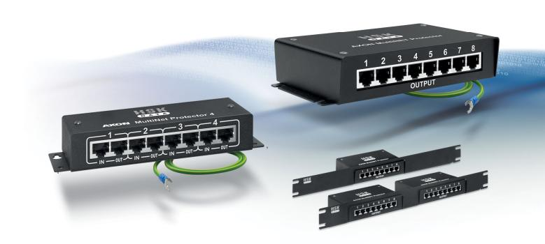
The **AXON Multi Net Protector** family of products is designed to protect against pulse surges, the 10/100/1000 Mb/s Ethernet appliances. The **AXON Multi Net Protectors** work with modems, routers, network cards and all other Ethernet network elements that use twisted pair cable terminated with RJ45 plug. They are multichannel devices dedicated to protect server rooms, local telecommunication networks and all other systems based on multiple lines.
