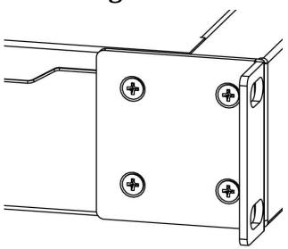
The device is designed to use indoors and it can be mounted in a rackmount enclosure using provided rack mounts, or it can be placed on the desktop. Please attach rubber pegs on the bottom of the router if the desired placement is on the flat surface or use a Phillips screwdriver to attach rackmount ears on both sides of the device if designated use is for rackmount enclosure:
