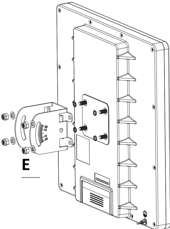
Now take the mounting bracket (E), and put it on to the back of the antenna. Use one rubber ring, one washer, and one nut for each of the built-in bolts (in that order).
